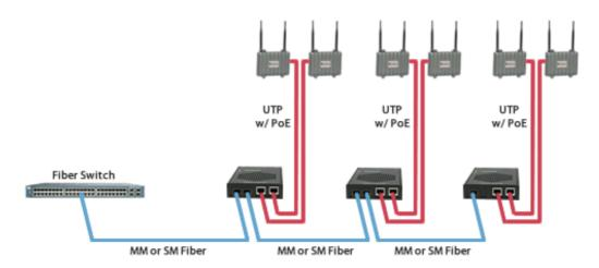
A second option is to have redundant fiber links for installations requiring fiber facility protection. There is an active fiber port and a protection fiber port that can support a fiber failure switchover of less than 50 milliseconds. The PoE+ media converter supplies power to the camera, and has power protection from an Uninterruptible Power Supply (UPS) battery back-up. In the event of a fiber cut and a loss of power, the camera continues to send data on the protection link.
